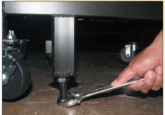
After adjusting the leveling feet, tighten the lock nuts. Also lock any casters that are resting against the floor after you have adjusted the leveling feet.
