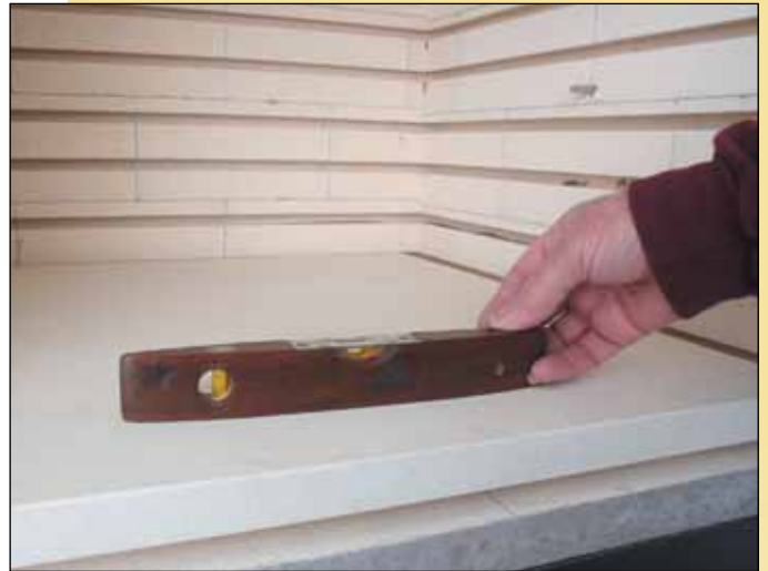
Place the level on the kiln shelf and take readings from several directions.
