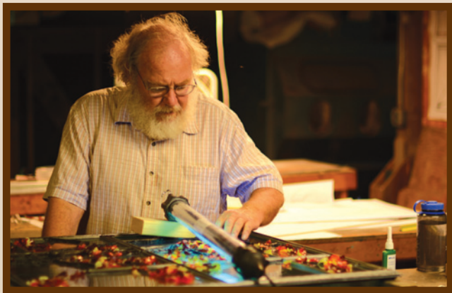
Wayne Cain assembling leaves on a window in progress. Photo by Will White.
