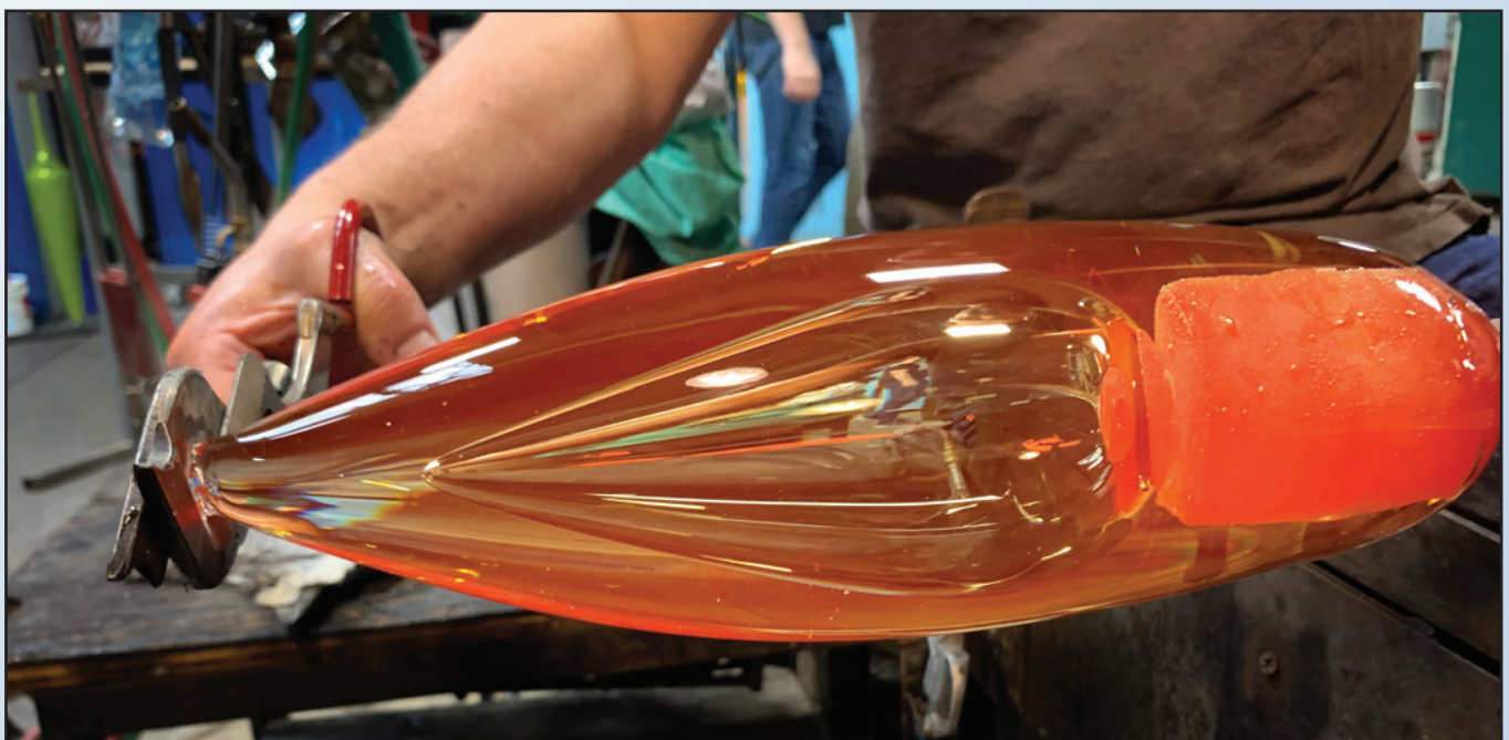
Stretching the bubble.
