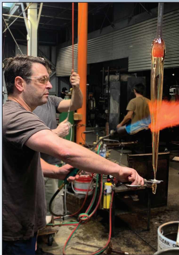
Pulling a point on the glass bubble.
