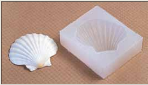
(Figure 3) Shell and corresponding flexible mold.
