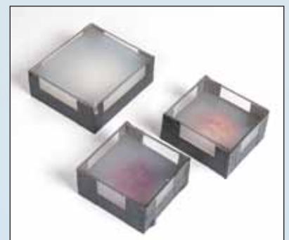
(Figure 2) Container filled with silicone rubber mold compound.
