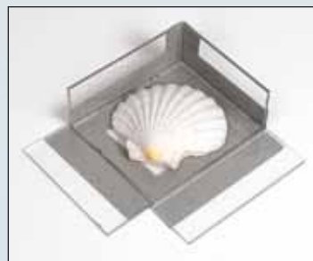
(Figure 1) Shell mounted with Plasticine™ in a glass box held together with duct tape.
