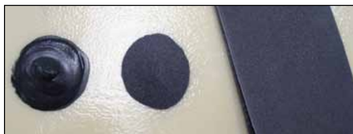
Silicon carbide in 120 grit is shown here in three forms: (left to right) slurry (wet grit), dry grit, and glued to paper backing (sandpaper).
