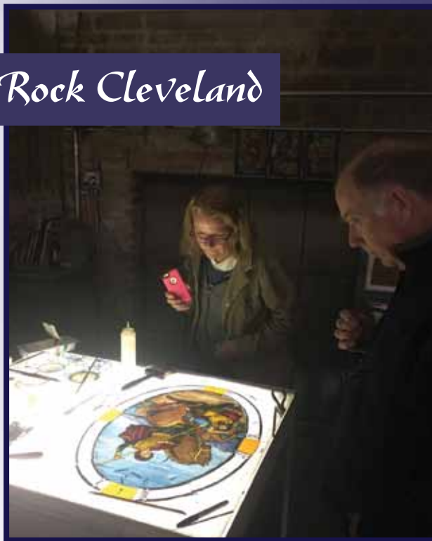
Cindy Courage and Rick Prigg examine a panel under construction at Whitney Stained Glass. Photo by Tony Glander.
