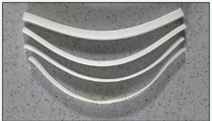
(Figure 2) For glass strips of equal span, the thicker the glass, the less the degree of slumping when fired simultaneously to the same temperature.
