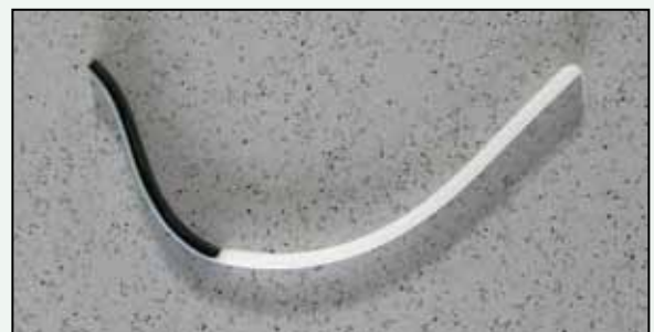
(Figure 4) The variation in viscosity from soft black glass to stiff white glass results in a lopsided slump.
