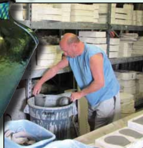
Gary Prusinski pouring slip for manufacturing the molds.
