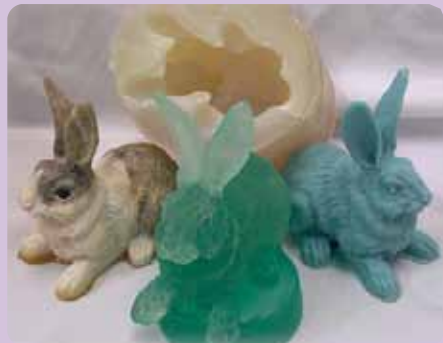
L-R: Original | Silicone Mold | Wax Pattern | Glass Casting Created with R&R GLASS-CAST 910 investment
