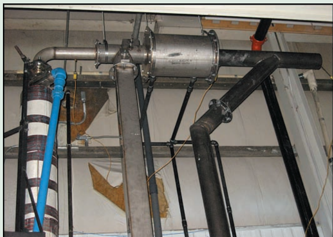
STARworks Glass furnace recuperator with diverter and heat exchanger.
