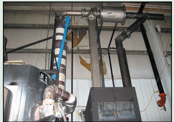
STARworks Glass furnace with recuperator, exhaust heat reclamation train and batch preheater.
