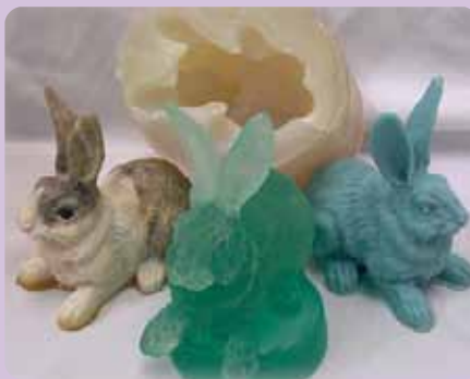
L-R: Original | Silicone Mold | Wax Pattern | Glass Casting Created with R&R GLASS-CAST 910 investment
