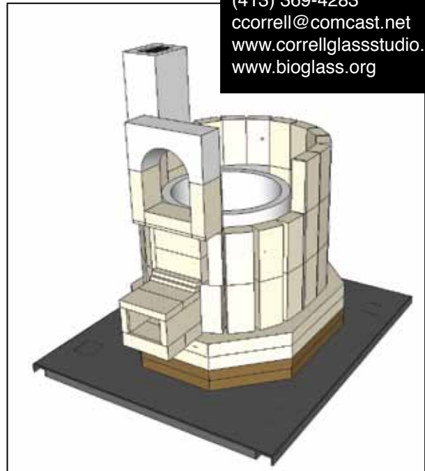
A CAD drawing of the 200-pound Pot Furnace as it would appear half finished.
