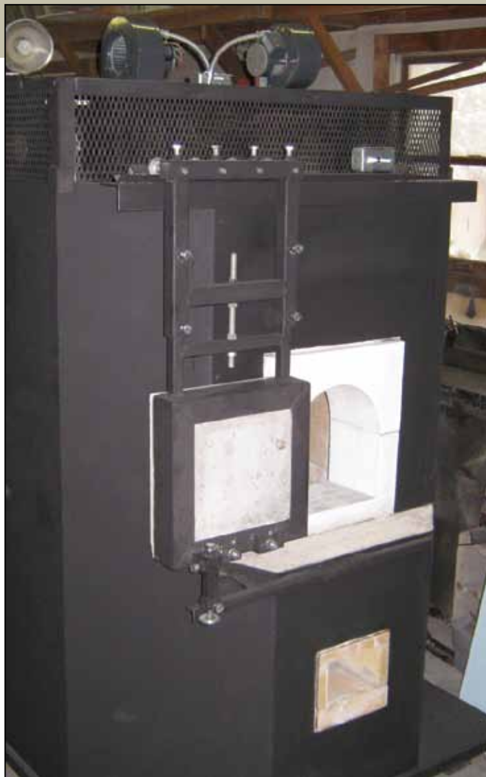
Completed electric "Moly" Furnace in Charles Correll's shop.
